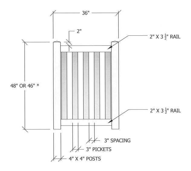
\* IF ADDITIONAL BOTTOM SWING CLEARANCE IS NEEDED, LIKE OVER A SIDEWALK, ORDER 46" GATE
