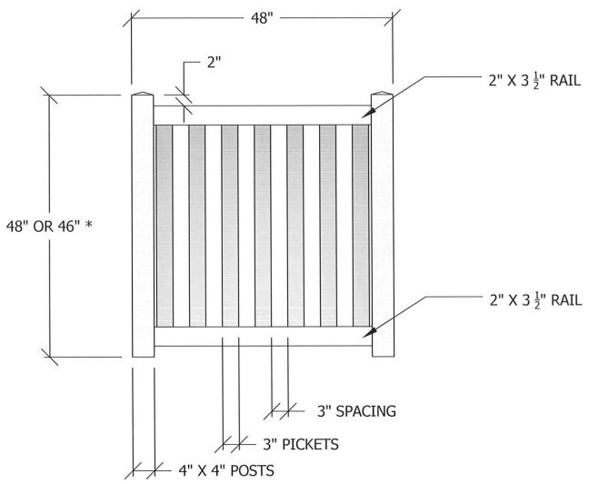
\* IF ADDITIONAL BOTTOM SWING CLEARANCE IS NEEDED, LIKE OVER A SIDEWALK, ORDER 46" GATE
