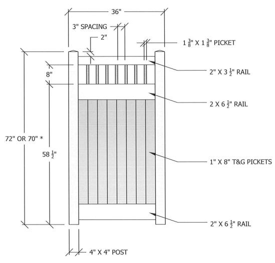
\* IF ADDITIONAL BOTTOM SWING CLEARANCE IS NEEDED, LIKE OVER A SIDEWALK, ORDER 70" GATE
