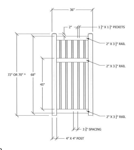
\* IF ADDITIONAL BOTTOM SWING CLEARANCE IS NEEDED, LIKE OVER A SIDEWALK, ORDER 70" GATE
