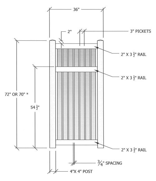
\* IF ADDITIONAL BOTTOM SWING CLEARANCE IS NEEDED, LIKE OVER A SIDEWALK, ORDER 70" GATE
