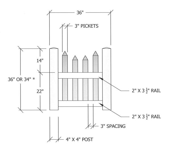
\* IF ADDITIONAL BOTTOM SWING CLEARANCE IS NEEDED, LIKE OVER A SIDEWALK, ORDER 34" GATE
